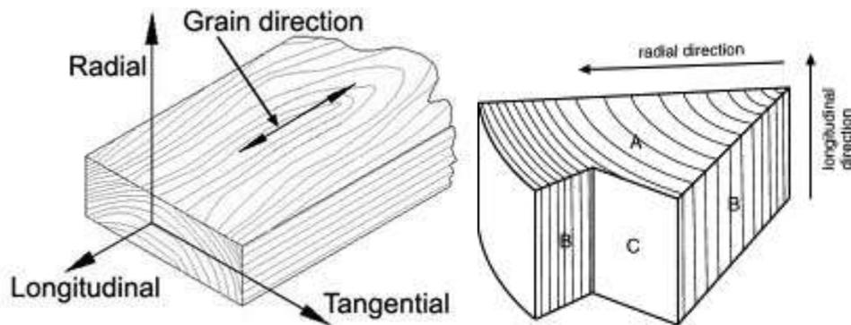
**Figure 1: Grain Direction Definition for Wood Structure**
