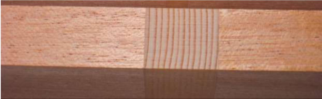
**Figure 2: Test Sample: Radial Grain Loading Direction**
