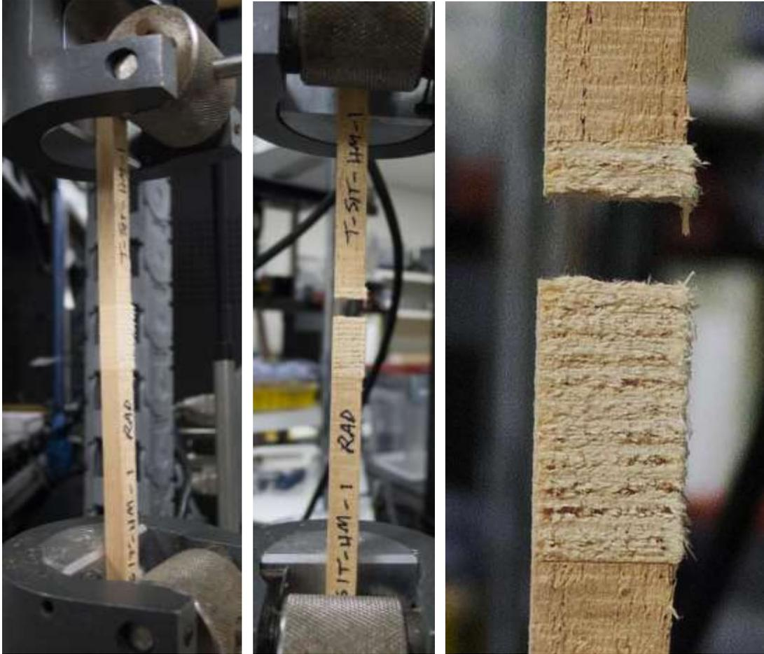
**Figure 8: Radial Specimen Under Test – Typical Failure**
