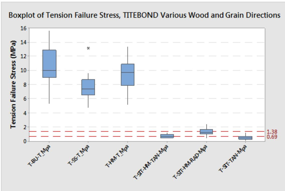
**Figure 6: All Tensile Results for Titebond Compared**
