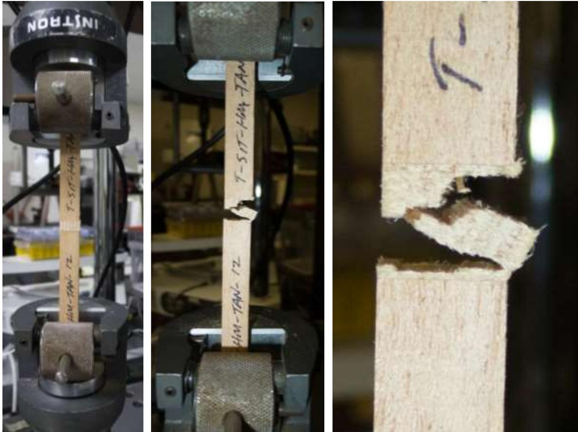
**Figure 7: Tangential Specimen Under Test – Typical Failure**
