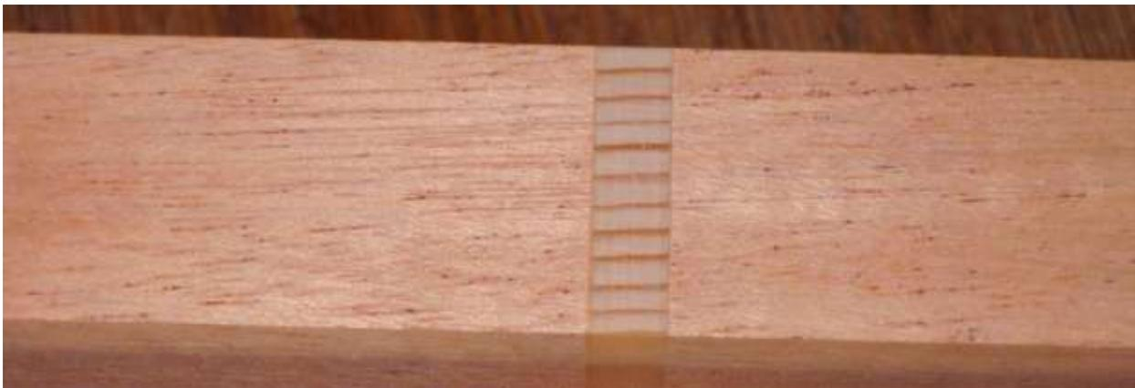
**Figure 3: Test Sample: Tangential Grain Loading Direction**
